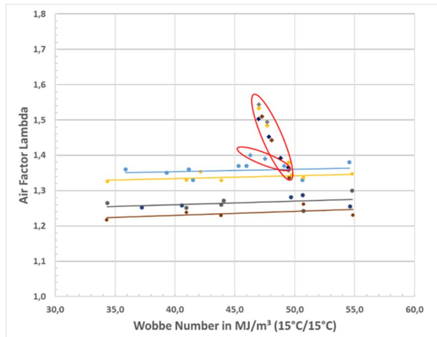
Figure 5 Measurement results from 4 boilers equipped with ionization sensors to monitor air/gas ratio
