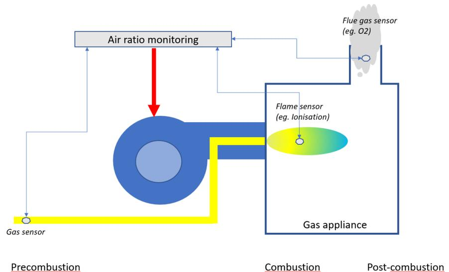
Figure 1 Principle of air ratio monitoring with different options
